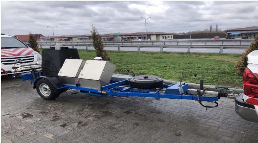
Figure 1. Equipment for strength assessment by the FFWD method [2]
