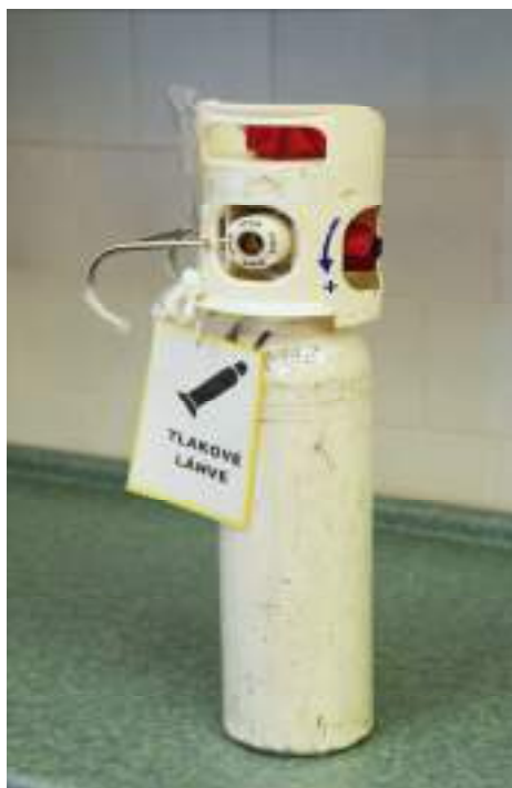
Fig. 16-3: Oxygen cylinder with integrated valve (LIV)
