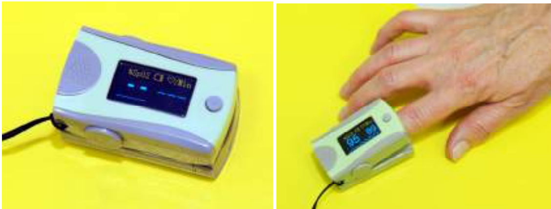
Fig. 16-6: SpO 2 and pulse measuring with pulse oximeter
